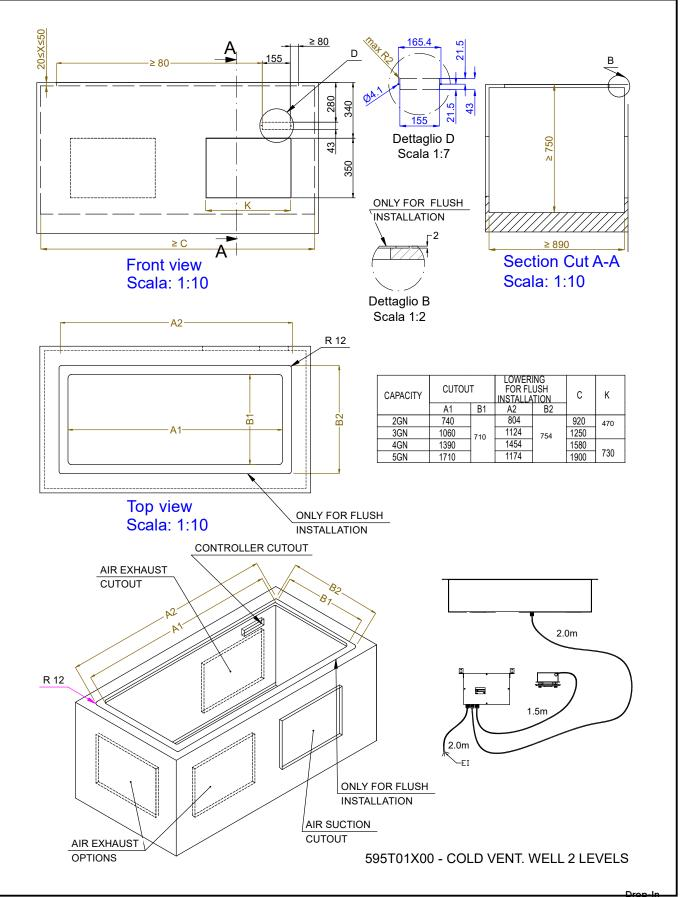
Drop-in Drop-in refrigerated well, ventilated, 1 refrigerated shelf and 1 neutral shelf (2 GN) The company reserves the right to make modifications to the products without prior notice. All information correct at time of printing.
