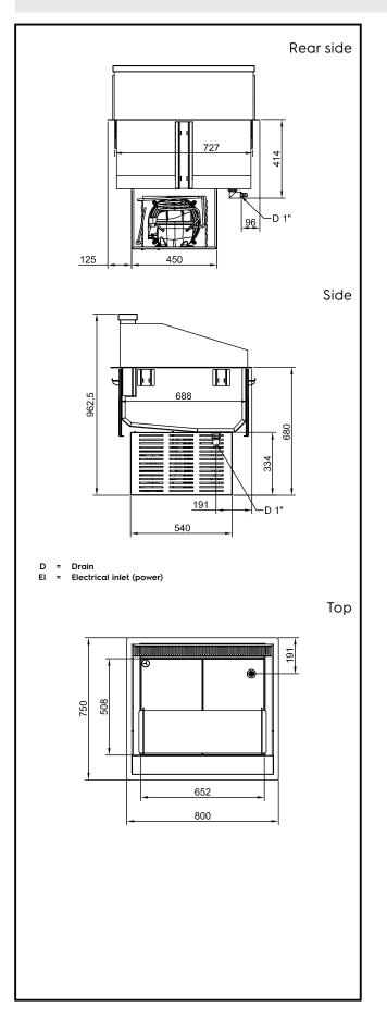
Drop-In Drop-in refrigerated well, ventilated, 1 refrigerated shelf and 1 neutral shelf (2 GN) The company reserves the right to make modifications to the products without prior notice. All information correct at time of printing.
